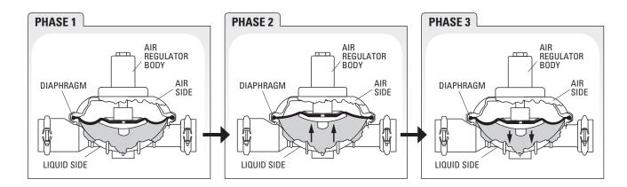
A compressed air line attached to the air regulator body sets and maintains pressure on the air side of the diaphragm. As the reciprocating pump begins its stroke, liquid discharge pressure increases which flexes the Equalizer® diaphragm inward. This action accumulates fluid in the liquid chamber (see Phase 2) and the air regulator allows compressed air to enter the air side. When the pump redirects its motion
