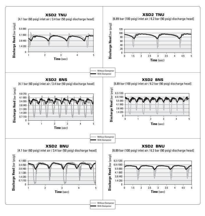
These charts show discharge head fluctuations for a diaphragm pump with and without a dampener. By reviewing the variation in pressure, the level of dampening can be estimated for an application. For example in reference to XSD2 BNS 100/90, the head pressure generated by a 51 mm (2") pump operating at 6.89 bar (100 psig) air inlet pressure and 6.2 bar (90 psig) head pressure
